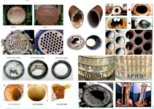
Areas to be cleaned and descaled using D'Scale 1000 and D'Scale 3000.
